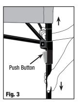
HANDY TIP: To fully engage the push button, grip the top and bottom frame members and squeeze as shown in Fig. 3A. Be careful to avoid pinch points.
